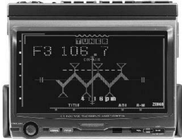
1-DIN HEAD UNIT, AM/FM/CeNET CD CHANGER CONTROLLER, 6.4" ACTIVE MATRIX COLOR LCD DISPLAY
