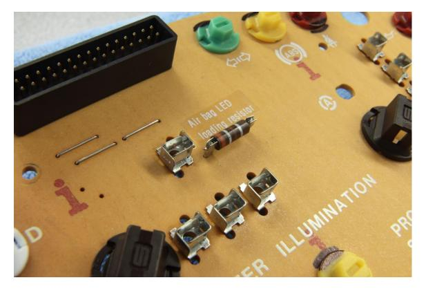
Figure 18: Added 390  $\Omega,$  ½ W loading resistor in parallel to air bag LED lamp
