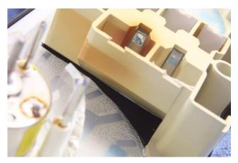
Figure 16: Black tape added to help prevent analog gauge backlighting from bleeding into A/T selector lever position indicators
