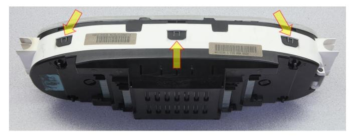
(Figure 8 and Figure 9 show the back of the cluster still attached; yours is probably removed at this point.)
