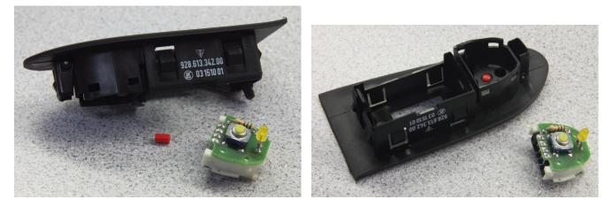
If you wish to bench test the LED backlighting, just apply 12 V to the terminals (the top two in the photo) as shown in Figure 22.
