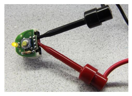
Figure 22: Terminals for testing intensive windshield washer switch backlighting
