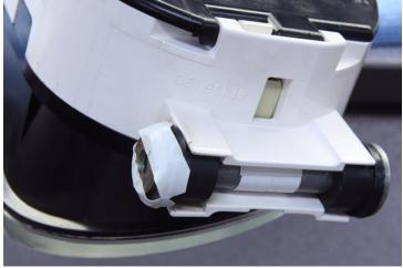
Figure 20: Taping the spacers, bushings, and washer
