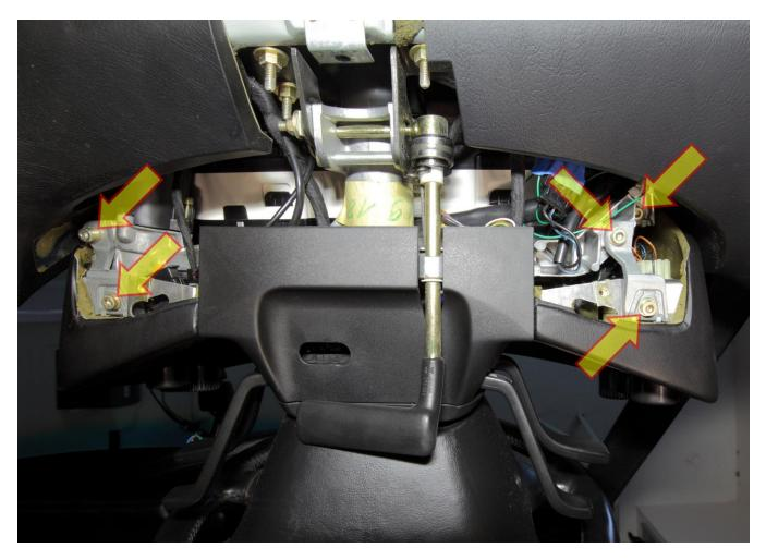
Figure 2: Looking up at the bottom of the instrument pod and the five screws that secure it
