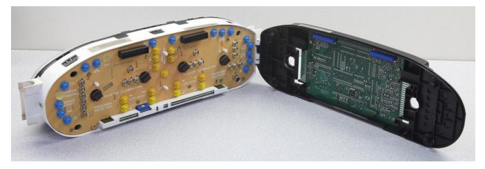
If you open them up all the way (about 90°) as shown in the above photo, the two pieces will completely separate at the hinge when you move the white half up and the black half down.
