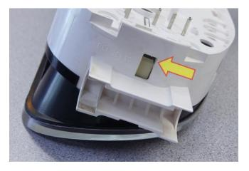
Figure 10: Slot to use for prying the front part from the center part of the cluster
