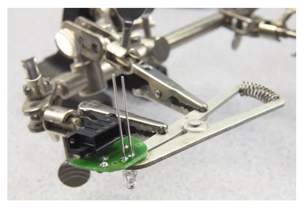
Figure 23: Soldering the replacement LED to the intensive windshield washer switch module (cathode on right)
