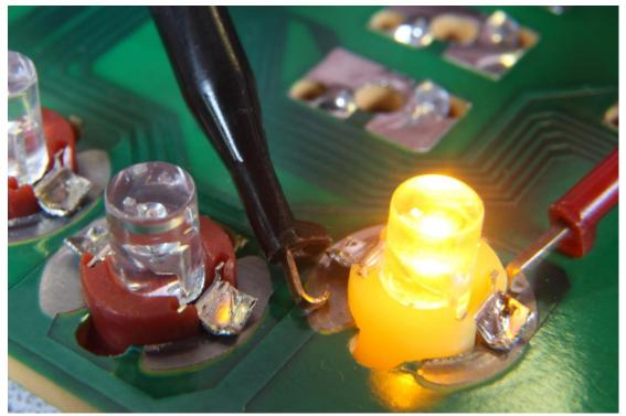
Figure 7: Testing B8.4d LED lamp "in-circuit"
