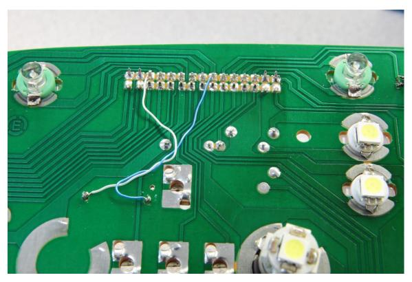
Figure 19: Connections for air bag LED loading resistor; solder wires as shown
