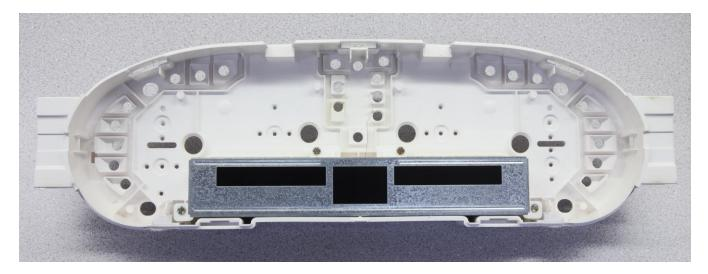
Figure 12: Center part of instrument cluster
