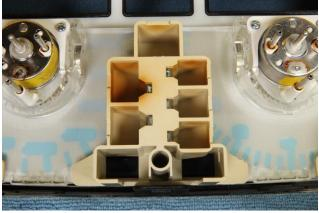
Figure 13: A/T selector lever position indicator bulb housings before modification
