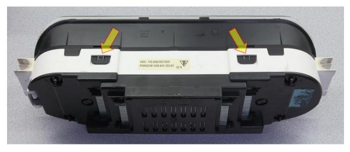
Figure 9: Two front-part-to-center-part-of-cluster latching fastening tabs on the bottom of the cluster
