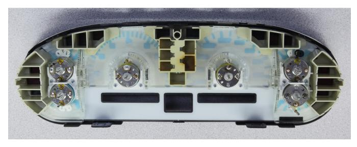
Figure 11: Front part of instrument cluster (be careful with this: it is fragile and will further separate into two pieces very easily!)
