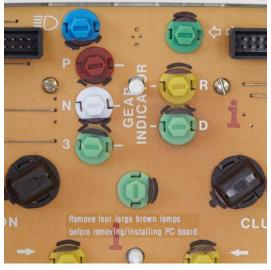
Figure 6: Alternative A/T bulb color scheme
