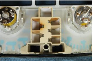
Figure 14: A/T selector lever position indicator bulb housings after white tape added to improve reflectivity
