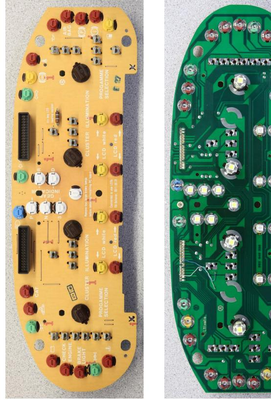
Figure 21: Back and front of PC board after LED replacement; black marks Indicate LED cathode (low/ground) side
