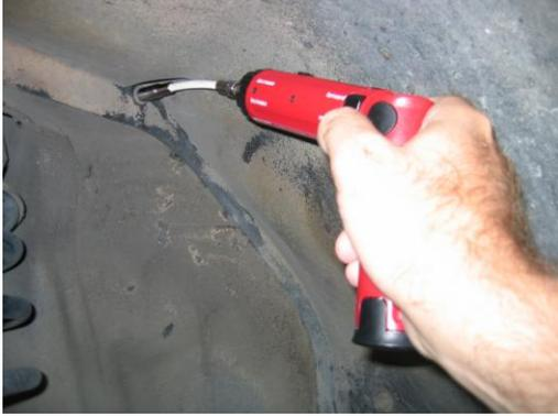
3. Remove top semicircular wheel well liner. There are three 8 mm hex-head screws, three 10 mm hex-head screws, and one 10mm hex-head plastic nut/washer. This is a good time to use an electric screwdriver and flexible extension, if you're so equipped. Once you've got all the fasteners out, you might be surprised how much you need to wiggle, twist, and pull on it to get the liner out.
