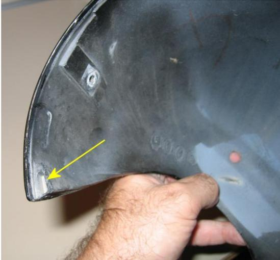
**Note:** when you replace your headlight covers, make sure you get the small oval indentations (the arrow in the photo on the left points to the left one, and there is another identical one on the right side) to fit over the small metal pins. These two pins secure the bottom of the headlight cover. If you don't do this correctly, the corner of the cover will be floppy and pushed away from the headlight.
