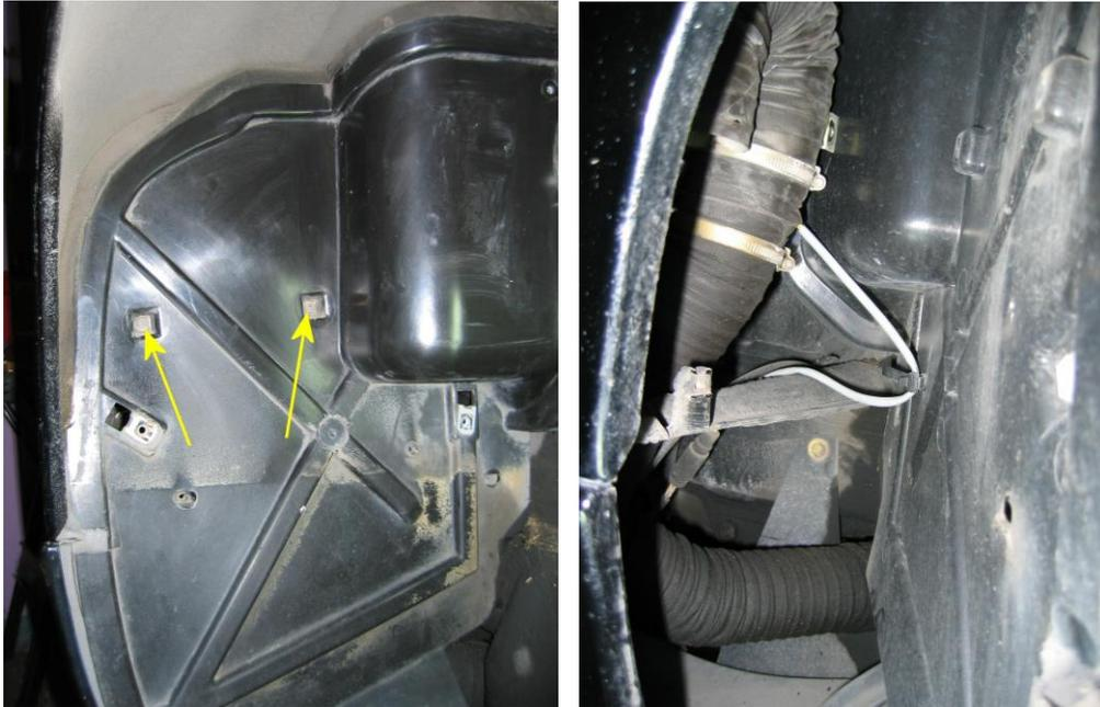
When you get the liner loose, you will also need to unfasten a cable holder on the other side that fastens a cable to the temperature sensor that lives inside the alternator cooling hose.
