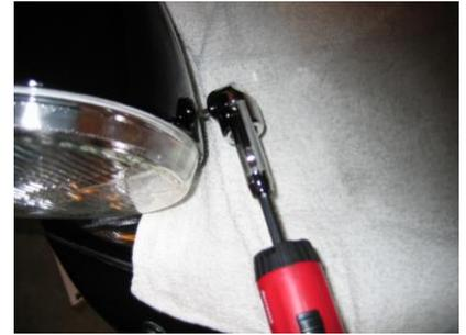
6. **{Headlight Up, Headlight Arm Down}** Unplug the H4 connector from the back of the headlight. Unscrew cable clamp #1 (Figure 10 ⑦) and cable clamp #2 (Figure 10 ⑧). Pull the cable/connector from the top to the bottom of the headlight assembly through the passageway (Figure 10 ⑨) and leave it dangling for later use.
