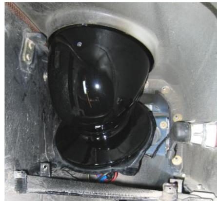
**{Headlight Down, Headlight Arm Down}** — This is the normal headlights down and off position. On the '90 S4, if the headlight switch is in the off position “0”, the headlights are usually down. If they're not (because the ignition switch was previously turned to the off position while the headlights were up), they can be put down again by just turning the ignition switch to the accessories position “1” momentarily until the headlights go down and then back to off position “0”.
