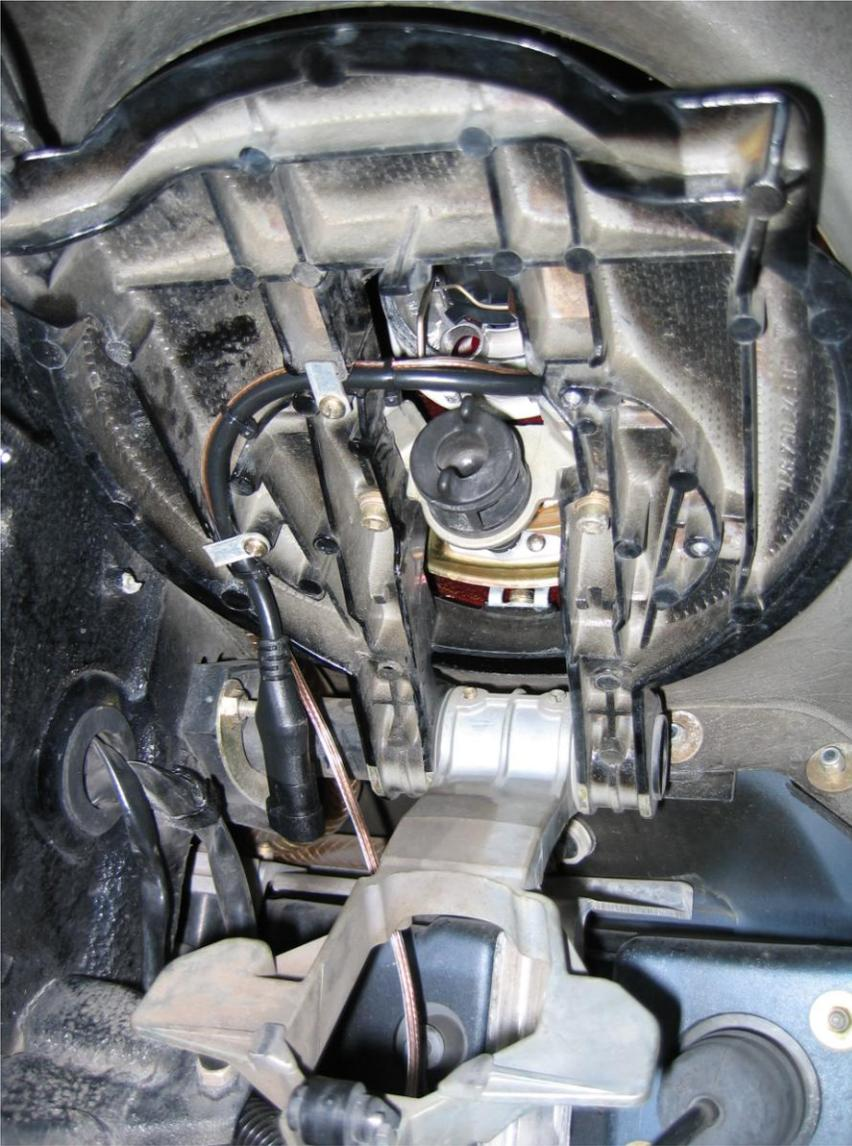
**Figure 12 Routing the Cables from Top Side of Headlight to Bottom Side**
