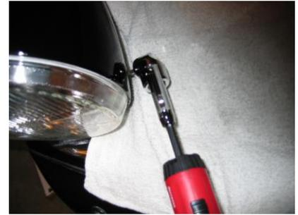
6. **{Headlight Up, Headlight Arm Down}** Unplug the H4 connector from the back of the headlight. Unscrew cable clamp #1 (Figure 10 ⑦) and cable clamp #2 (Figure 10 ⑧). Pull the cable/connector from the top to the bottom of the headlight assembly through the passageway (Figure 10 ⑨) and leave it dangling for later use.
