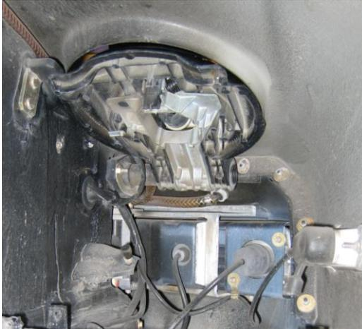
**{Headlight Up, Headlight Arm Up}** — On the '90 S4, you can stay in this state with the actual lamp turned off by: (a) turning headlight switch to full on position “2”, (b) turning ignition switch to the accessories position “1” momentarily until the headlights pop up, (c) turning ignition switch to the off position “0”, (d) turning headlight switch to off position “0”.
