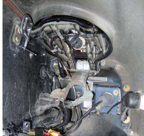
**{Headlight Up, Headlight Arm Down}** — This is an abnormal state, but can be achieved (when you have access to the area under the headlight assembly) by clamping the headlight assembly to the upper stop, even when the headlight arm is down. It is safe to move the headlight shaft and arm while the headlight is clamped like this, as long as there are no other obstructions in the path of the headlight arm.
