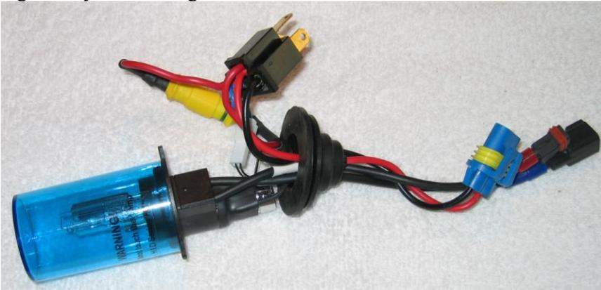
Use scissors and cut the grommet off, being very careful so you don't cut or nick the wires. You can leave a couple of little pieces to hold the remaining pairs of wires together, as shown below.
