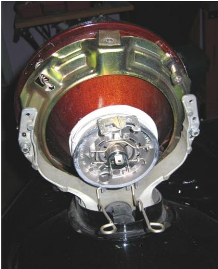
7. Remove the weather seal — if your headlight has one — (Figure 9 ⑥) from the back of the headlight assembly by squeezing together the retaining clip (Figure 9 ⑤) to release it, flipping it out of the way, and then lifting/peeling away the weather seal. Set the weather seal aside; you will not be able to reuse it with the HID bulb (unfortunately).
