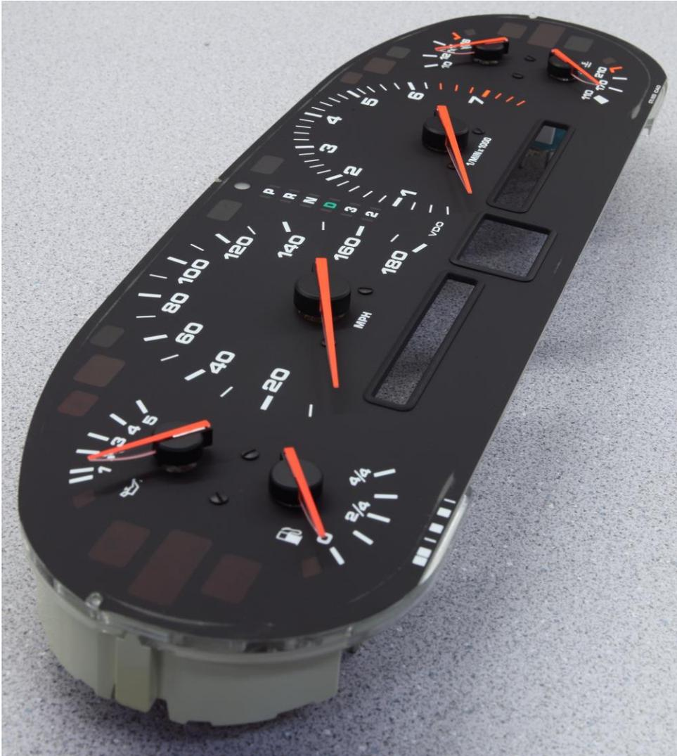
Figure 17: Analog gauges, freed from their housing
