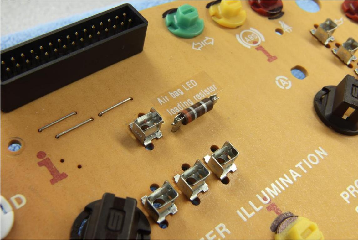
Figure 18: Added 390  $\Omega$ , 1/2 W loading resistor in parallel to air bag LED lamp
