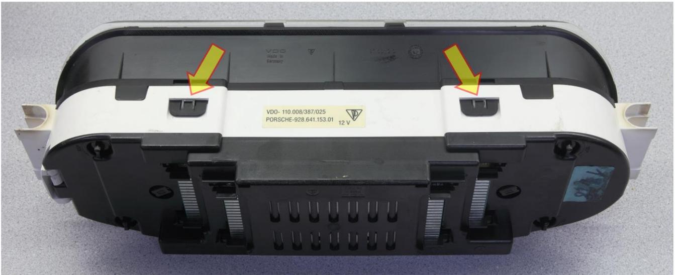
Figure 9: Two front-part-to-center-part-of-cluster latching fastening tabs on the bottom of the cluster
