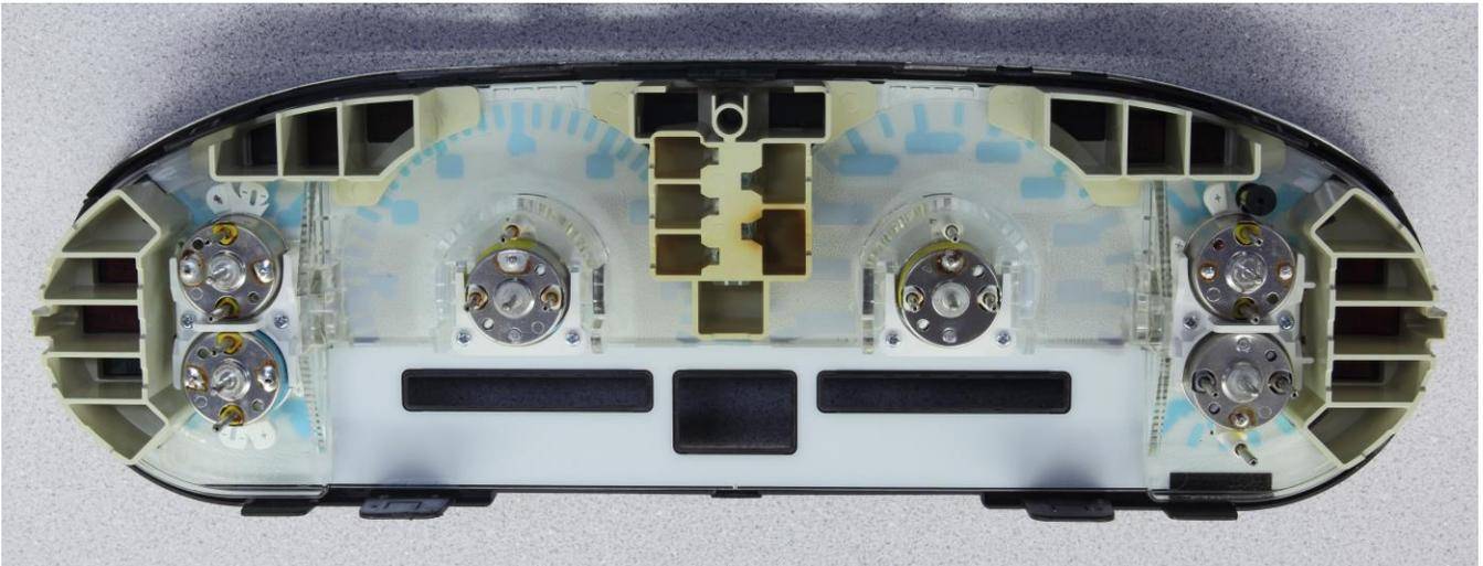
Figure 11: Front part of instrument cluster (be careful with this: it is fragile and will further separate into two pieces very easily!)
